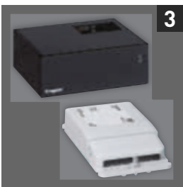
Supervisory controller and Wi-Fi access point
