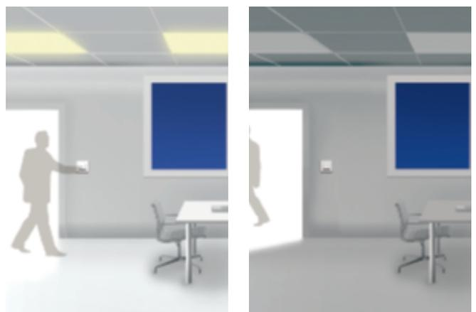
Upon entering the room the person switches on the light as normal, but on leaving the sensor switches off the lighting automatically. Lights can also be switched off manually.
