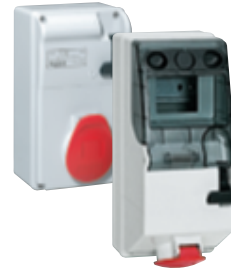
SINGLE-SOCKET UNITS With or without DIN rail: 16 / 32 A IP 44 et 63 A IP 66 (see page 25)
